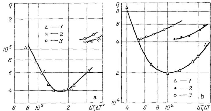
Fig. 4. Dependence of the thermal load on the difference between the surface temperature of the coating and the saturation temperature of the liquid (a: water): 1) sphere without coating; 2) specimen No. 4 in coordinates  $q-T$ ; 3) specimen No. 4 in coordinates  $q-\Delta T'$ ; (b: Freon-113): 1) sphere without coating; 2) specimen No. 1 in coordinates  $q-\Delta T$ ; 3) specimen No. 1 in coordinates  $q-\Delta T'$ .  $\Delta T$ ,  $\Delta T'$ ,  $^{\circ}C$ .
