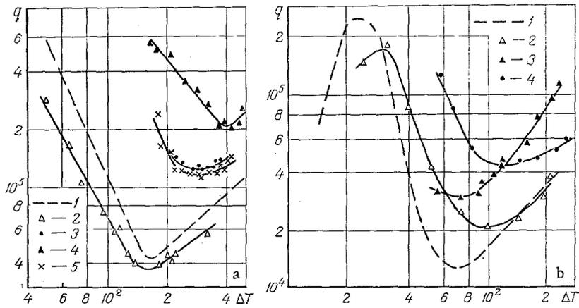
Fig. 3. Dependence of the thermal load on the difference of the temperature of the sphere and the saturation temperature of the liquid (a: water): 1) plate without coating [9]; 2) sphere without coating; 3) specimen No. 2; 4) No. 3; 5) No. 4; (b: Freon-113): 1) plate without coating [9]; 2) sphere without coating; 3) specimen No. 1; 4) No. 5.  $q$ ,  $W/m^2$ ;  $\Delta T$ ,  $^{\circ}C$ .
